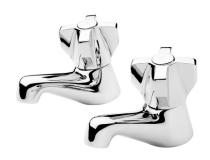
PBT1 PRODUCT CODE Chrome COLOUR/FINISHES All Pressures PRESSURE TYPE 17kPa MIN. PRESSURE MAX. PRESSURE 500kPa (As per NZ Building Code AS/NZ 3500.1) WELS RATING Low/Unequal 2 Star; 11.5L/min Mains 3 Star; 8.5L/min MAX. TEMPERATURE 65°C PLUMBING CONNECTION 15mm Non Rising Headwork - FORPT65 REPLACEMENT PART/S Handle - FORPT217
