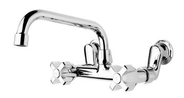
PSF4 PRODUCT CODE COLOUR/FINISHES Chrome All Pressures PRESSURE TYPE 17kPa MIN. PRESSURE MAX. PRESSURE 500kPa (As per NZ Building Code AS/NZ 3500.1) Low/Unequal 4 Star; 7L/min **WELS RATING** Mains 3 Star; 9L/min MAX. TEMPERATURE 65°C PLUMBING CONNECTION 15mm Non Rising Headwork - FORPT65 REPLACEMENT PART/S FORPT05 - Universal Sink Faucet Spout Primus Handle - FORPT42 15mm Offset - FORPT45 Adjustable Offsets - 100 to 230mm WALL FIXINGS
