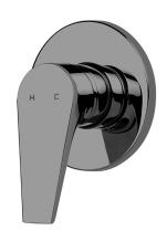
**SLT30MB** PRODUCT CODE Black/Chrome COLOUR/FINISHES White/Chrome Mirrored Black (PVD) Chrome PRESSURE TYPE All Pressures 35kPa MIN. PRESSURE MAX. PRESSURE 500kPa (As per NZ Building Code AS/NZ 3500.1) 65°C MAX. TEMPERATURE PLUMBING CONNECTION 15mm FACEPLATE DIAMETER 117mm CERTIFICATION Watermark
